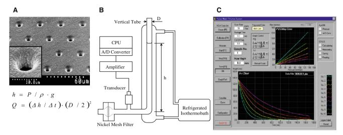
Fig. 1 a Scanning electron microscopic photograph of a nickelmesh-filter. Magnification of a single pore in nickel-mesh shows the smooth transition into the pore interior (*inset*). **b** Schematic illustration of gravity-based, nickel-mesh-filtration system. Height of the meniscus within the vertical tube (h) was obtained by continuous reduction of filtration pressure (P), specific gravity ( $\rho$ ), and
